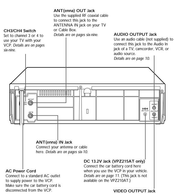
Use a video cable (not supplied) to connect this jack to the Video In jack of a TV, camcorder, VCR, or audiovisual source (laser disc, video disc player, etc.). *Details are on page 10.*
